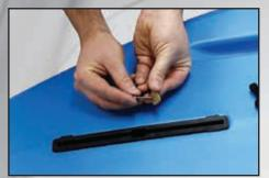
1- Clean the fin box to make sure it's free of debris. Insert the screw in the metal plate.
